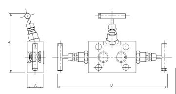
The 'Y34' and 'YV34' Type 3 valve manifolds are designed for direct mounting to differential pressure transmitters, with separate isolation for LP and HP inlets plus equalising valve for simple calibration. Each needle valve head is designed for safe and reliable isolation, giving bubble tight shut off, with non-rotating & antigalling tip and dynamic self-adjusting spindle seal to give long service life in a variety of service conditions.
