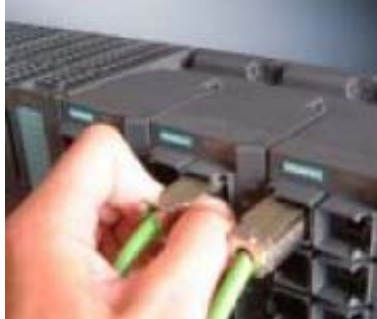
Figure 6-4 Releasing the RJ-45 Plug
