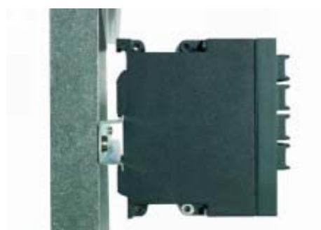
Figure 5-1 IE Switch X-200 removing from a DIN rail (35 mm)
