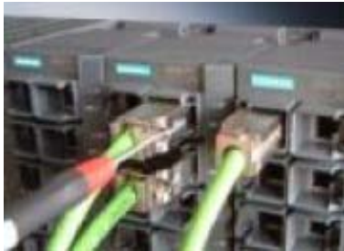
Figure 6-5 Releasing the RJ-45 Plug with a screwdriver
